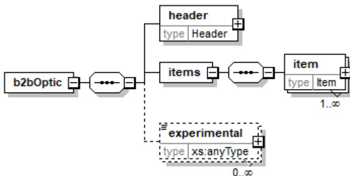
In the root-element the location of the XSD at schema.b2optic.com must be set, so the receiver could identify the version of XML.
